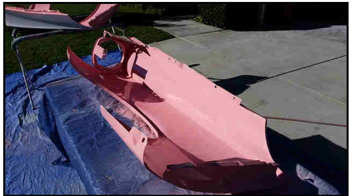
Inside the fenders painted.
